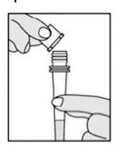
Tear off the top seal of the extraction vial with the enclosed opener.
