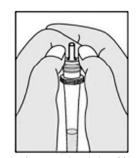
Firmly attached the filter nozzle to the top of the exxtraction vial.
